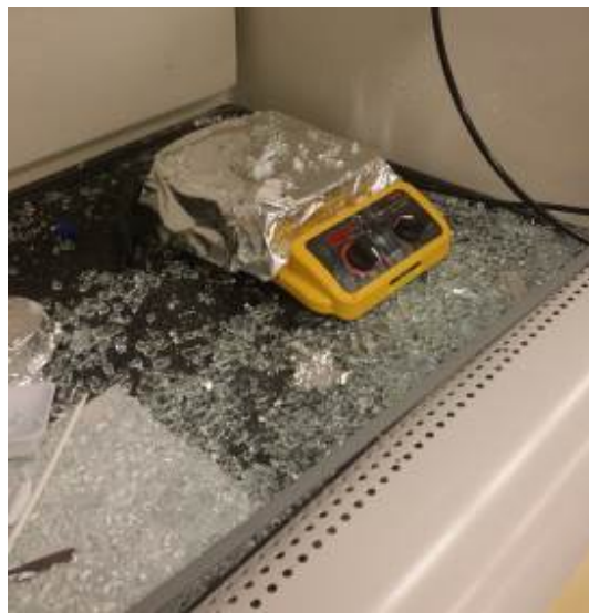
Over pressurization and Splutter of 50ml Lab Bottle
