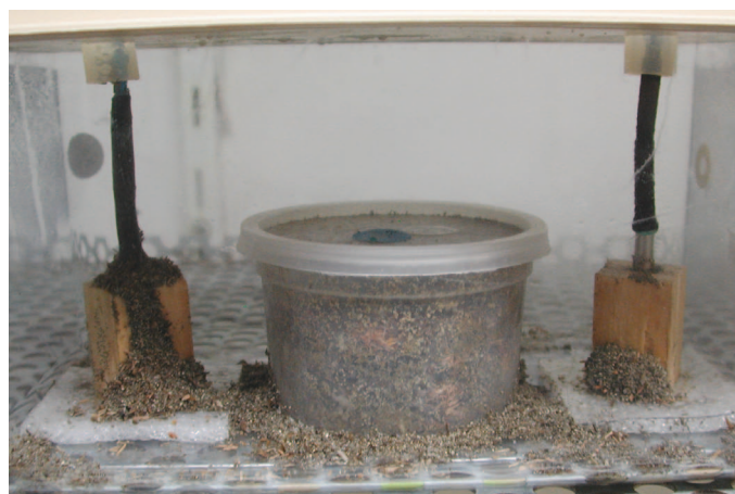
Termites attack wooden blocks according to vibration signals
